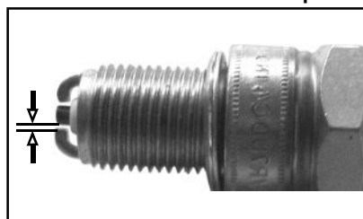
Double Electrode Spark Plug Gap
