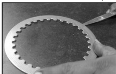
Clutch steel plate : Distortion
