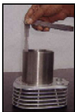
Piston ring end gap : compression rings
