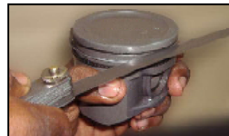
Ring to groove clearance : Comp. Top ring
