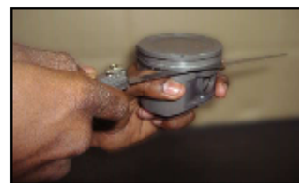
Ring to groove clearance: Comp. ring - Middle
