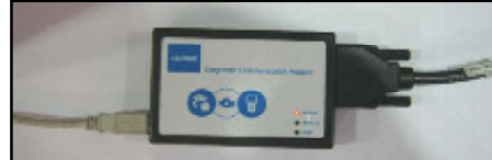
Communication Adaptor (A link between ECU & Computer System)
