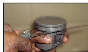
Ring to groove clearance : Oil rings
